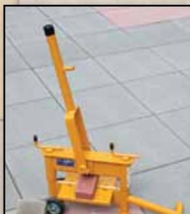
Handle shown in upright position. When adjusting height, always put the handle in the upright position.
