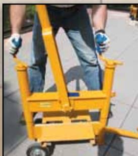
Adjust both height adjustment handles at the same time. If the screw towers bind up, adjust one side to make level before proceeding.
