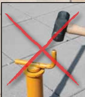
Never use a hammer or other mechanical device to operate height adjustment handles.
