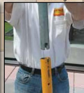
Insert extension handle to engage locking pin. Twist clockwise to lock
